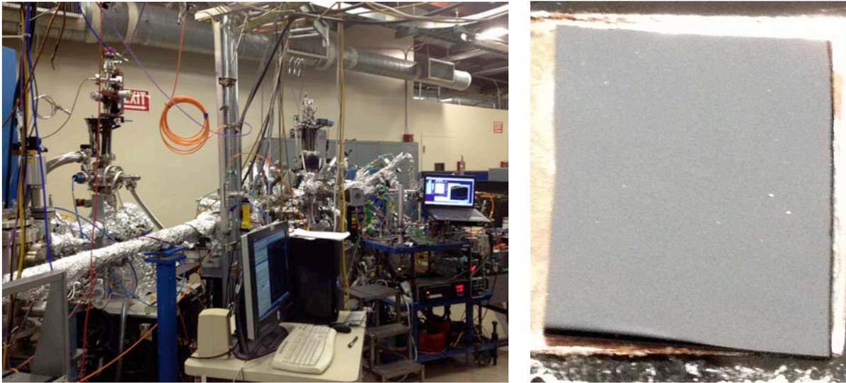
**Figure 6:** (Left) A photograph of the XPS experimental setup at SSRL that is used for surface characterization measurements. The setup has been recently upgraded for measurements of graphene samples. (Right) A piece of a silicon wafer coated with 10-nm-thick layer of alumina using ALD tool at SNF. The white dots show the marks left by the probe station tip during electrical characterization.
