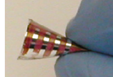
CNT based solar cells could be flexed to beyond 5mm radius of curvature with no ill effects, while ITO based cells splintered at these flexing angles.
