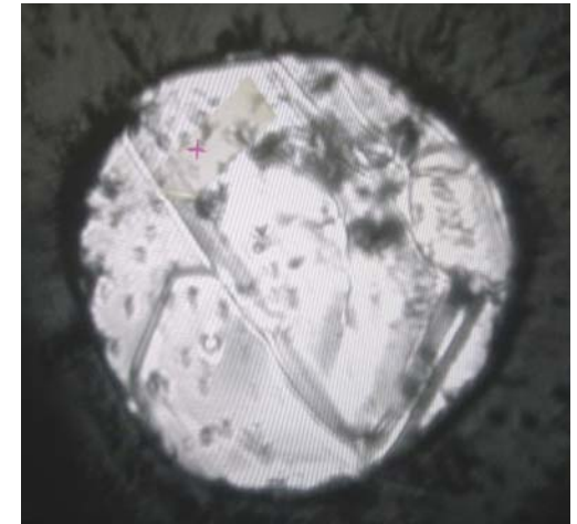
\text{CH}_4(\text{H}_2)_4 crystals at 3 GPa and 150 K
