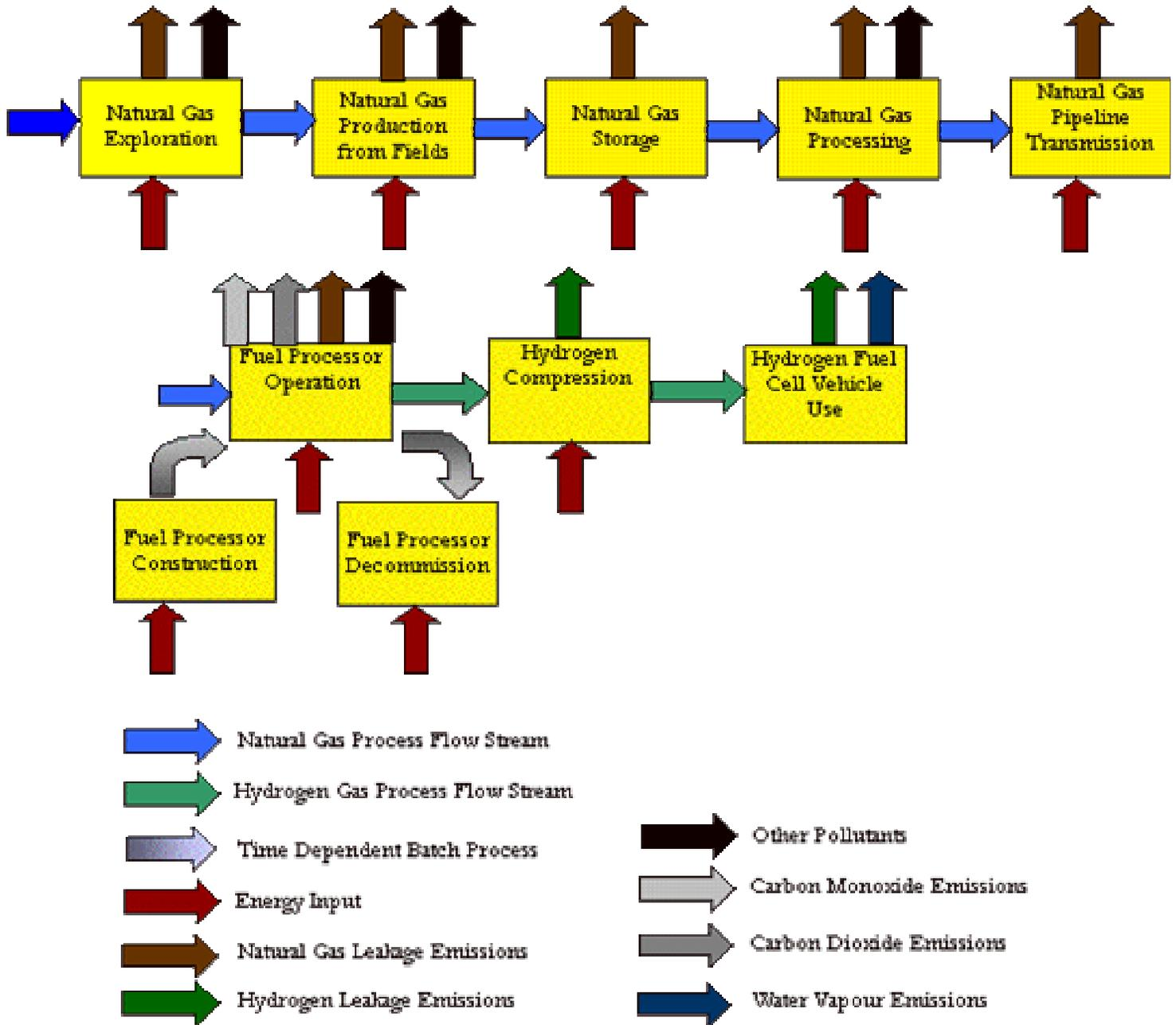
**Figure 1.** Process Chain Analysis of mass, energy, and pollutant flows in a scenario where hydrogen is obtained from natural gas.
