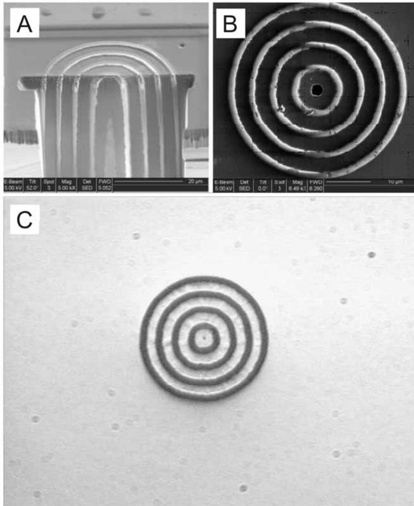
**Figure10:** A 40µm-diameter ETWI consisting of four 2µm-thick poly-silicon layers and four 1µm-thick thermal silicon-oxide layers A) SEM image of the cross section B) SEM image of the top view (poly-silicon and silicon appears as dark, silicon-oxide appears as bright) and C) Optical microscope image of the top view (poly-silicon and silicon appears as bright, silicon-oxide appears as dark).
