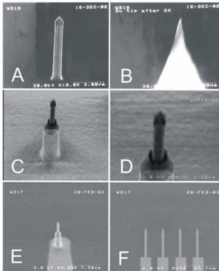
**Figure 3:** Tip-probes at different fabrication levels A) Example of an etched HARS tip B) Detail of a sharpened tip with a tip radius smaller than 50 nm C – D) HARS tips embedded in a 500 nm thick low stress silicon nitride E - F) Metallized embedded HARS tips.
