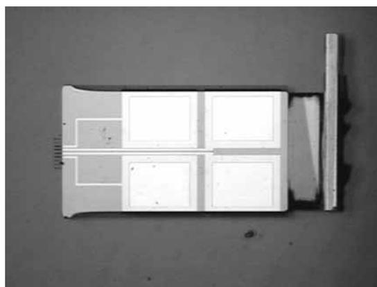
**Figure 5:** Optical low magnification micrographs of an SECM-AFM probe device.
