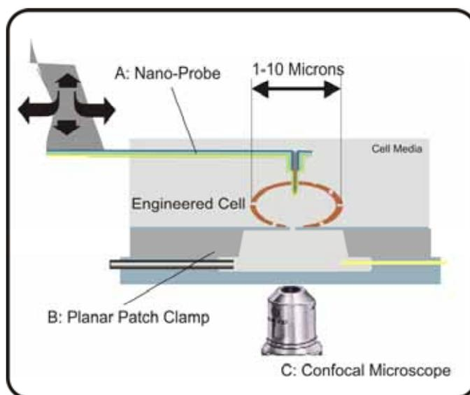
**Figure 1:** Single cell diagnostic platform with electrochemical nanoprobes, A: Electrochemical nanoprobes are mounted to an atomic force microscopic stage, B: Localization of single cells is achieved with a planar patch clamp device, C: For optical visualization a confocal fluorescence microscope is used.
