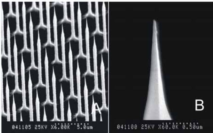
**Figure 9:** A) multi-array ultra sharp silicon tips fabricated with a combination of two plasma etching steps. B) a closer look of the individual silicon tip with a radius less than 20 nm
