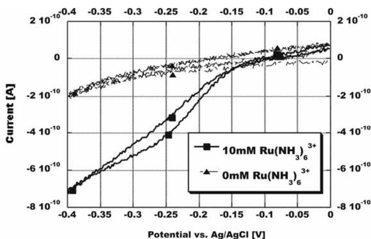
**Figure 7:** Cyclic voltammograms of tip probe with a platinum UEM ( $0.125 \mu\text{m}^2$ ) in 0.1 M Phosphate buffer electrolyte and in a 10 mmol  $\text{Ru}(\text{NH}_3)_6\text{Cl}$  and 0.1 KCl solution. The potential is related to a 0.1 M KCl Ag/AgCl-Reference electrode, Potential sweep rate was 10 mV/s.
