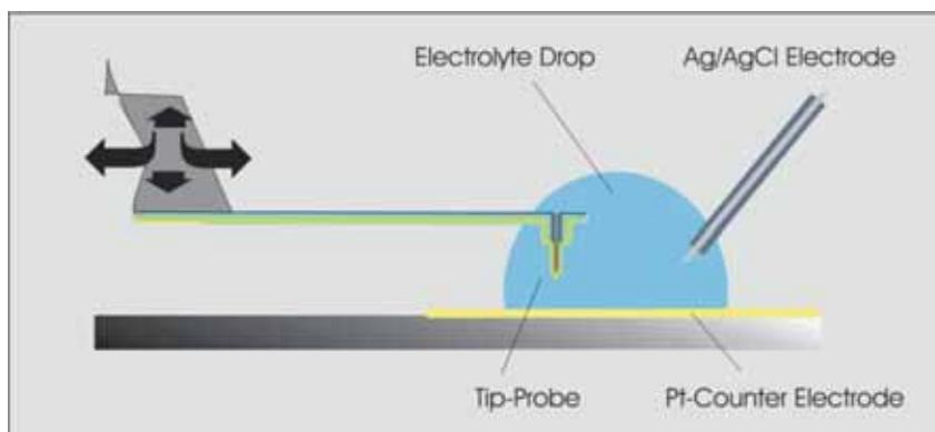
**Figure 6:** Schematic electrode arrangement of an electrochemical measurement set up.
