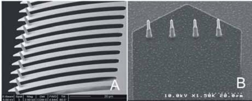
**Figure 8:** A) Silicon nitride cantilever array with single high-aspect-ratio tips. The thickness of cantilevers is about 500 nm B) High-aspect-ratio tip array on single silicon nitride cantilever.
