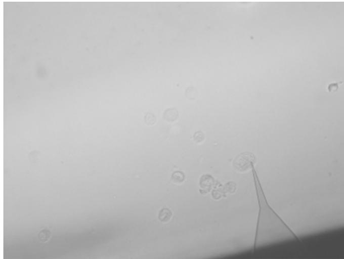
**Figure 11:** Ultra-sharp planer silicon nitride tip fabricated with a combination of micro-fabrication technique and FIB (Focused Ion Beam) techniques penetrating individual cells.
