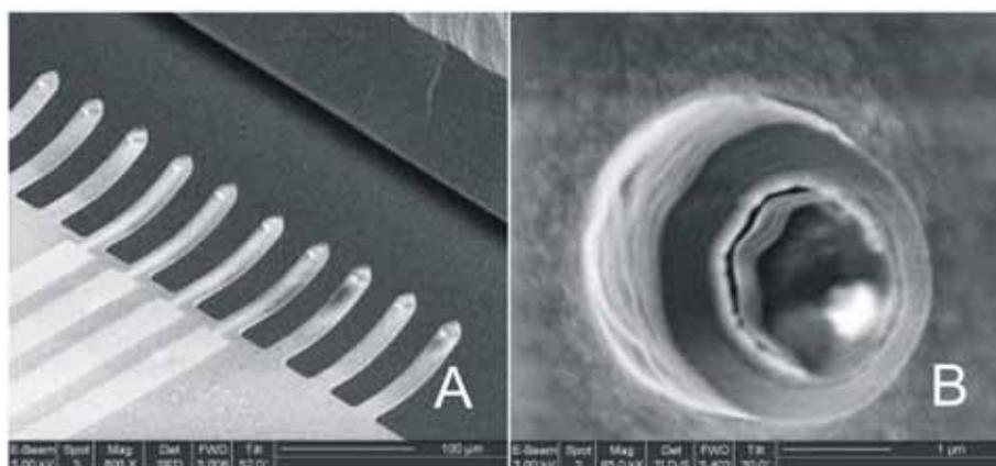
**Figure 4:** SEM pictures of a finished tip probe array A) Tip probe array with four UME cantilever structures B) Tip probe of the cantilever structures with a platinum UME (radius of  $200\ \text{nm}$ ).
