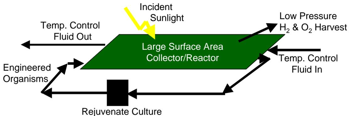
**Figure 2:** Diagram of a proposed production system for hydrogen production.
