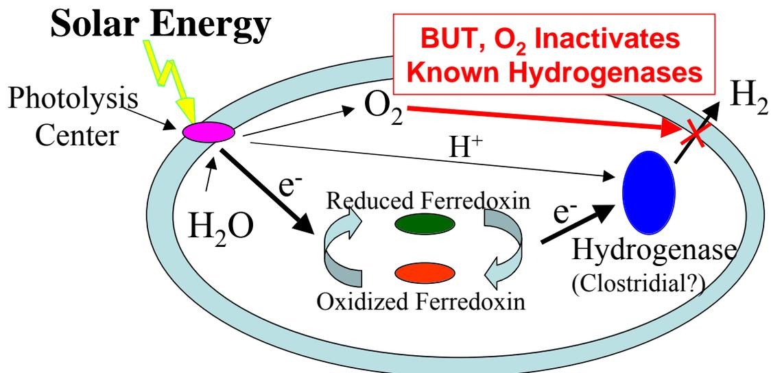
**Figure 1:** Diagram of proposed *Synechocystis* bacterium engineered to support a short, efficient pathway for the conversion of sunlight and water into molecular hydrogen. As shown, the dominant barrier to this technology is the availability of an oxygen-tolerant hydrogenase enzyme.
