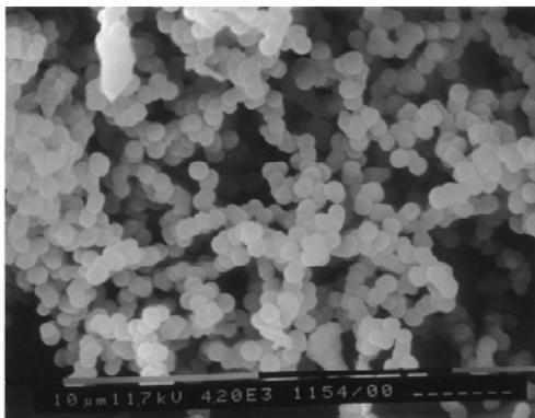
Figure 2. Scanning electron micrograph of a porous sol-gel polymer monolith (without enzyme).
