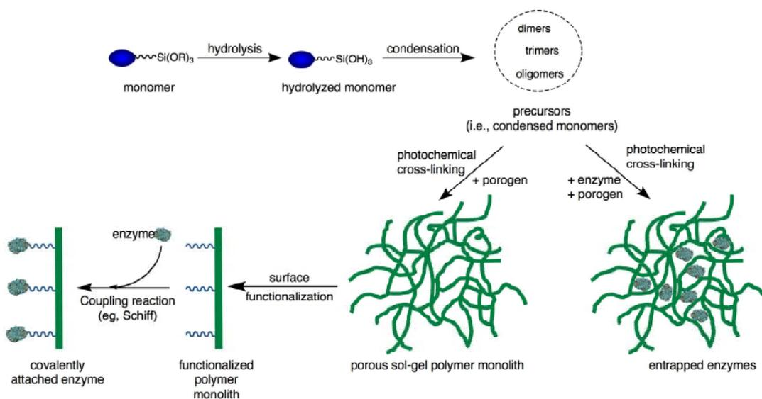
Figure 1. Schematic diagram of porous inorganic-organic sol-gel polymer preparation and immobilization of enzyme by covalent attachment and entrapment.
