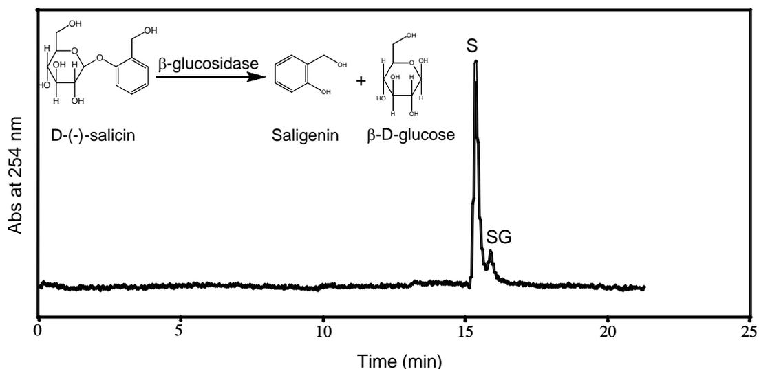
Figure 3. Separation of salicin (S) and saligenin (SG) after hydrolysis of salicin on a  $\beta$ -glucosidase enzyme immobilized in a sol-gel polymer monolith. Saligenin was formed after a 5-minute reaction with the immobilized enzyme.
