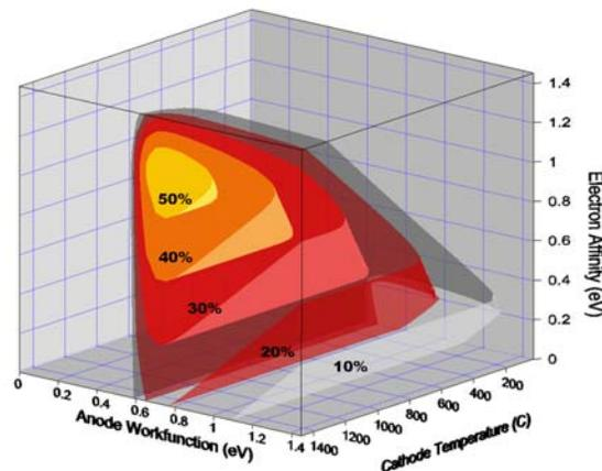
**Figure 3:** Theoretical PETE efficiency as a function of cathode temperature, anode work function, and cathode electron affinity.  $E_g$  is fixed at 1.4 eV, the number of collisions with the surface is  $10^4$ , and the anode temperature is 327°C.
